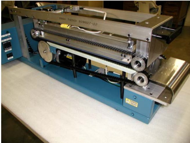
Direct Drive with Low Friction Idler Pulleys Left Side
