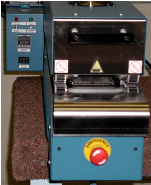
M175 Controls with E-Stop
